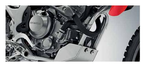
SKID PLATE 08P70-K1T-E50 (Only applicable on CRF300L)
